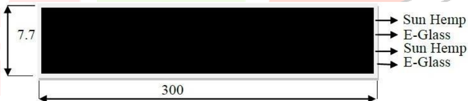
Figure 6 Sun Hemp 20% and E Glass 30% mould
