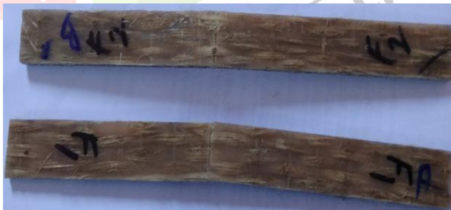
Fig. 9 Samples after flexural test
