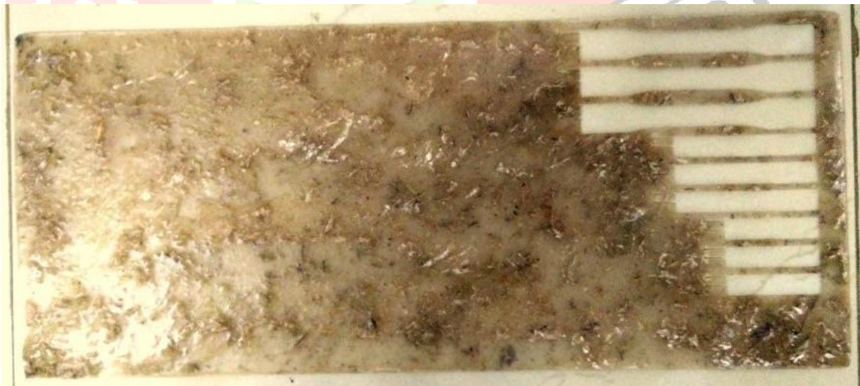
Fig 10 Composite sheet after water jet cutting
