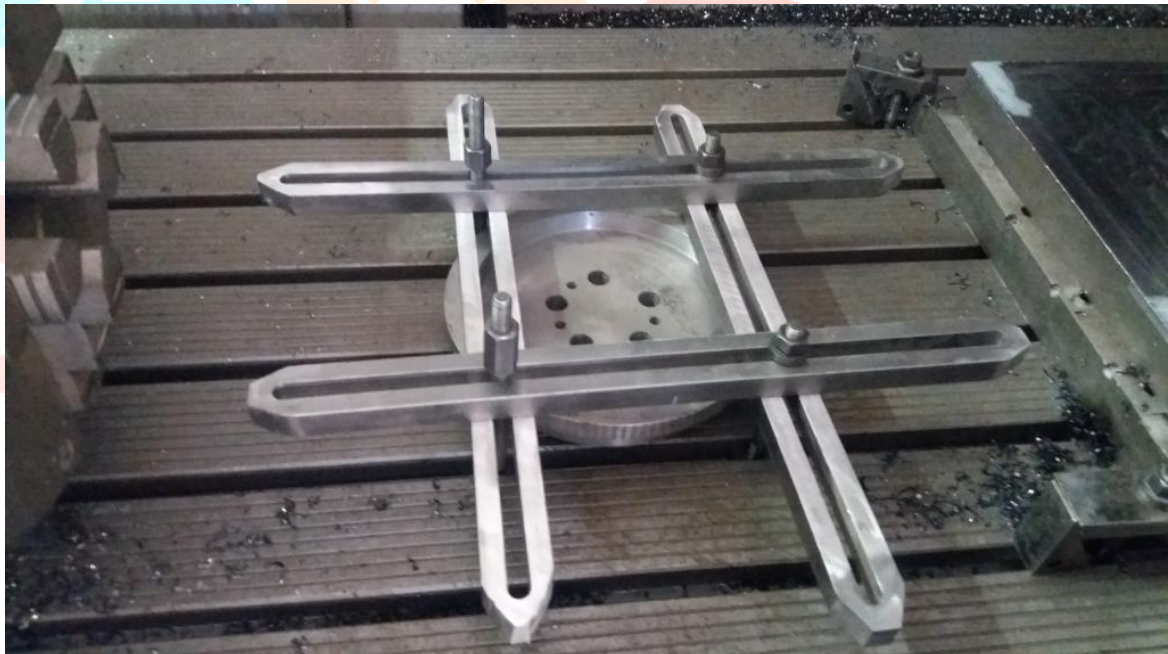
Fig.2 job 01 (Motor coupling cover)
