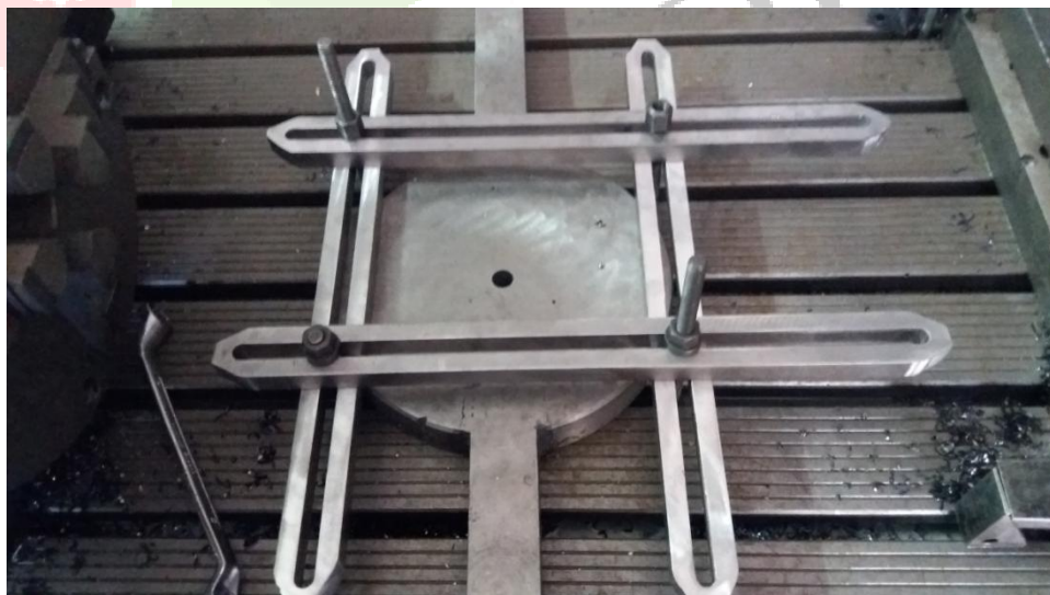
Fig.4job 03 (Slotted link)
