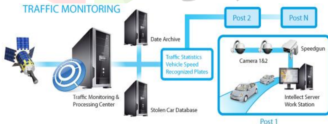
Fig 1. Block Diagram of Traffic Monitoring System [4]
