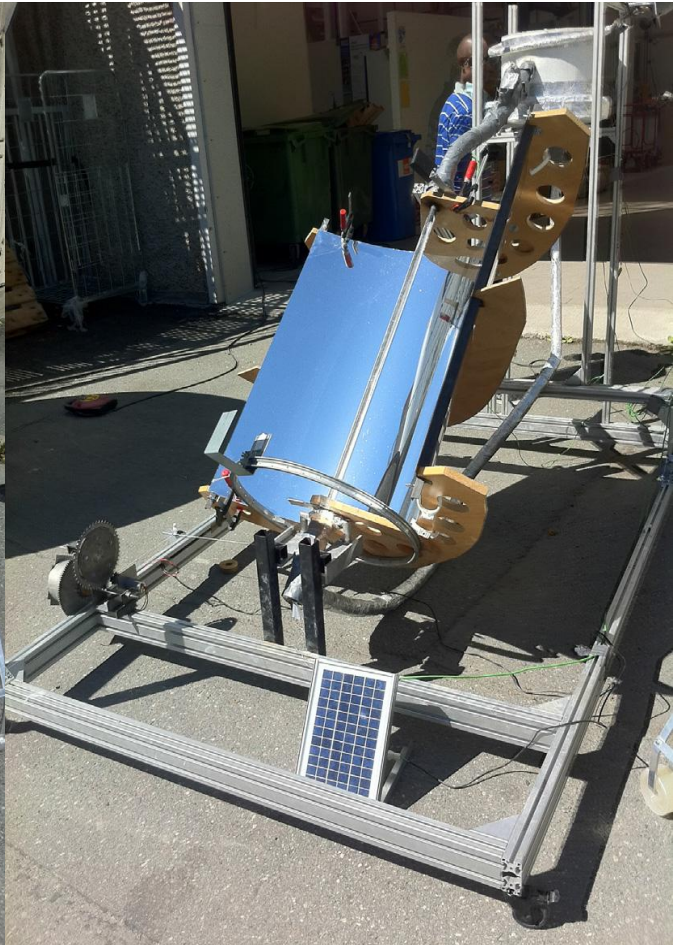
Fig. 7. Heat storage based system with parabolic trough [8]
