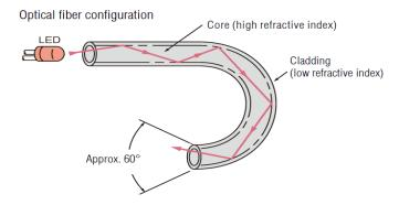
Significantly, the fiber optic technology has changed the advancement of telecommunication. Most of the components associated with these devices are often developed for the fiber-optic-sensor uses. The fiber optic sensors has increased the use in the place of traditional sensor. An optical fiber is a very thin fabril of plastic tube in which messages are transferred via light signals. These fabrils are bundled together in a protective cover and the whole assembly is known as fiber optic cable.
