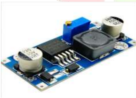
Figure.4. LM2596 Buck Converter
