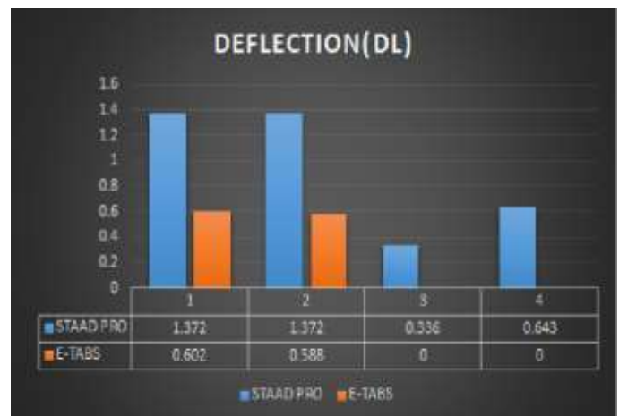
Graph 18 represents deflection (dl) in selected members of models 3.(All values are in mm).
