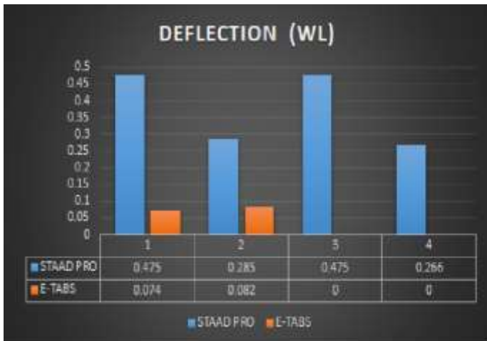
Graph 15 represents deflection (wl) in selected members of models 2.(All values are in mm).
