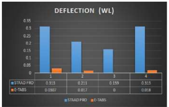
Graph 12 represents deflection (wl) in selected members of models 1.(All values are in mm).
