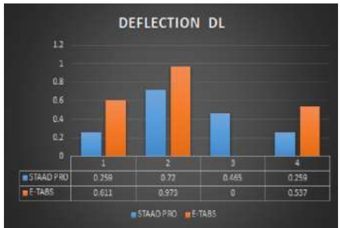
Graph 10 represents deflection (dl) in selected members of models 1.(All values are in mm).
