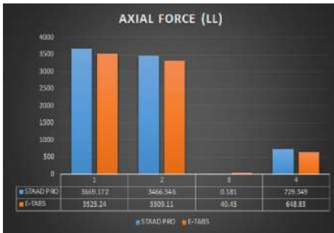
Graph 5 represents axial force (ll) in selected members of models 2. (All values are in kg).
