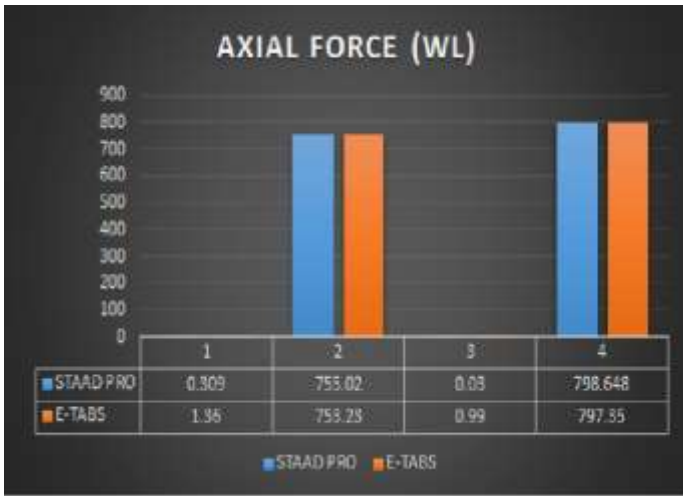
Graph 3 represents axial force (wl) in selected members of models 1. (All values are in kg).
