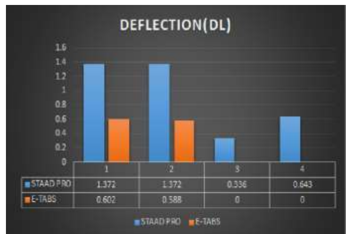
Graph 16 represents deflection (dl) in selected members of models 3.(All values are in mm).
