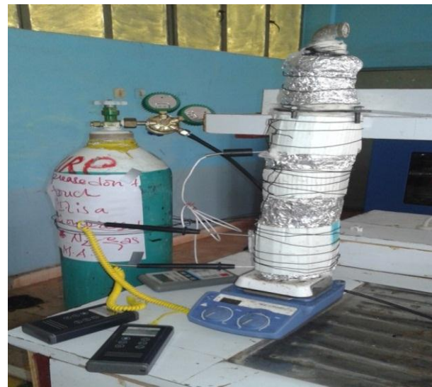
Figure 3: The actual experimental set up for torrefaction process
