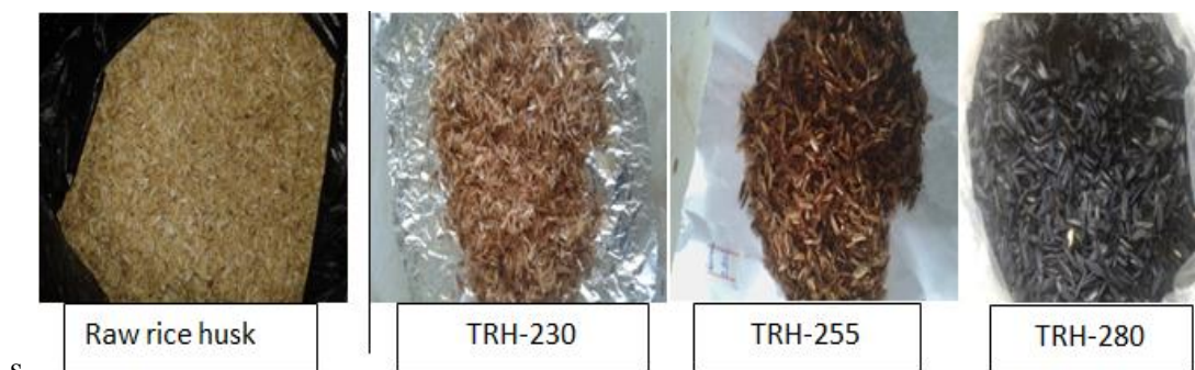
Figure 5: Effect of Torrefaction temperature on surface morphology of rice husk sample
