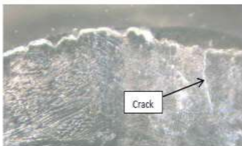
Fig: Crack yields in tensile test
