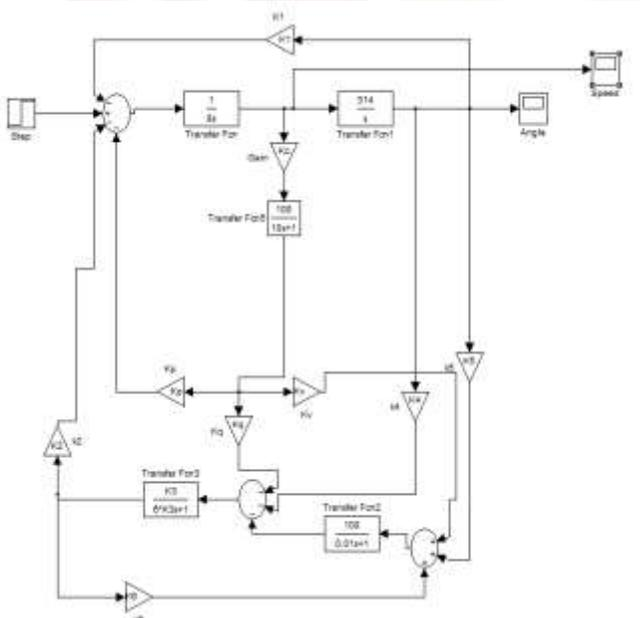
Fig.5: Simulink Model for SMIB power system with UPFC
