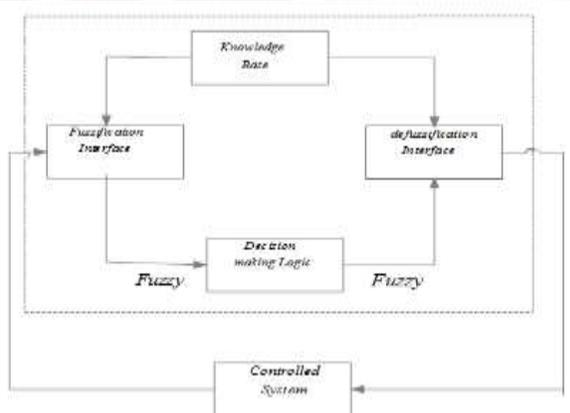
Fig.3. Basic structure of fuzzy controller
