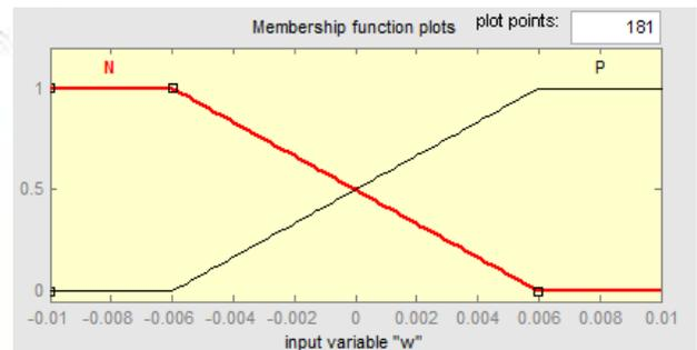
Fig. 4(a): Membership function of Error signal
