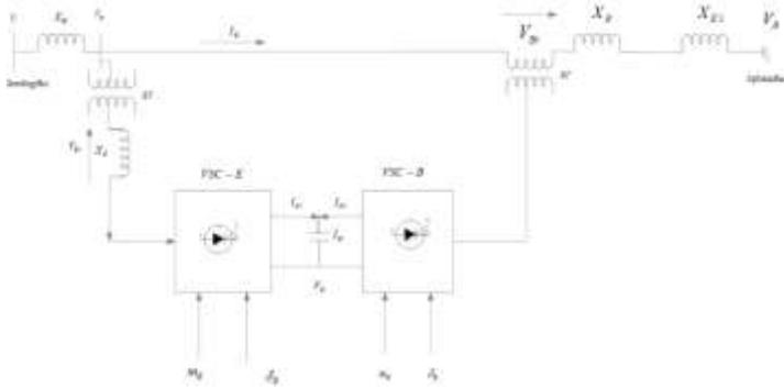
Fig.2 UPFC installed in SMIB system
