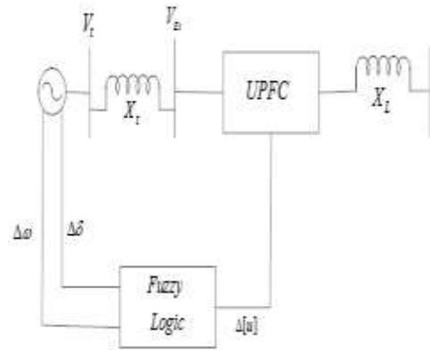
Fig.4: UPFC with Fuzzy logic controller
