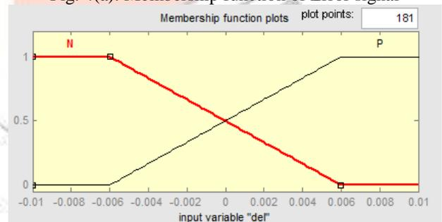
Fig. 4(b): Member function of Derivative signal
