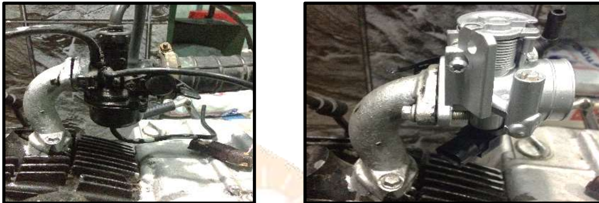
Figure 3 a. Existing fuel & air mixing and b. Modified Fuel & Air mixing
