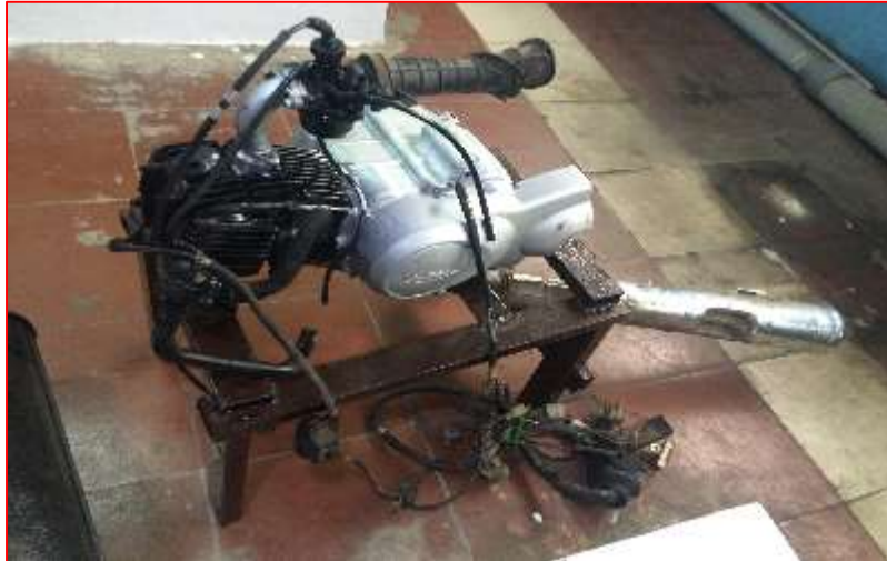
Figure 1 Air Cooled, 4 Stroke Single Cylinder OHC Engine.
