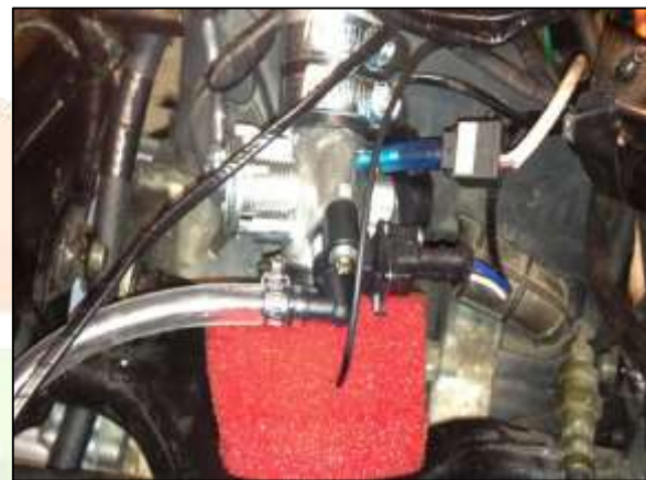
Figure 6 Engine Temperature Sensor & Intake Air Temperature Sensor Assembly
