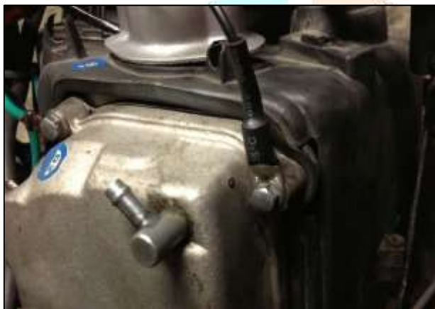
Figure 6 Engine Temperature Sensor & Intake Air Temperature Sensor Assembly
