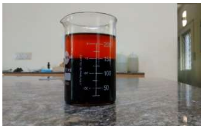
Fig.2 Biodiesel and glycerine formation by Trans esterification process
