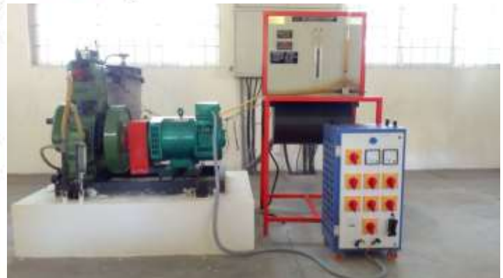
Fig.5 Single cylinder four stroke diesel engine with electrical dynamometer
