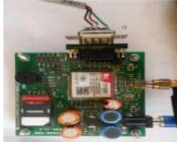
Fig 7.GSM SIM800.
