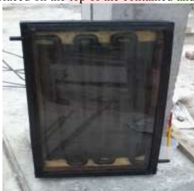
Fig.1: Fabrication of Solar Collector
