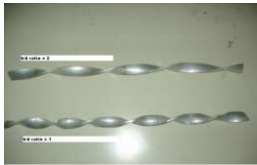
Fig.3.2: Twisted Tape Inserts
