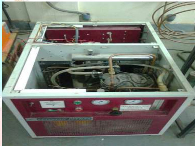
Fig. 3.5: Pictorial view of compressor
