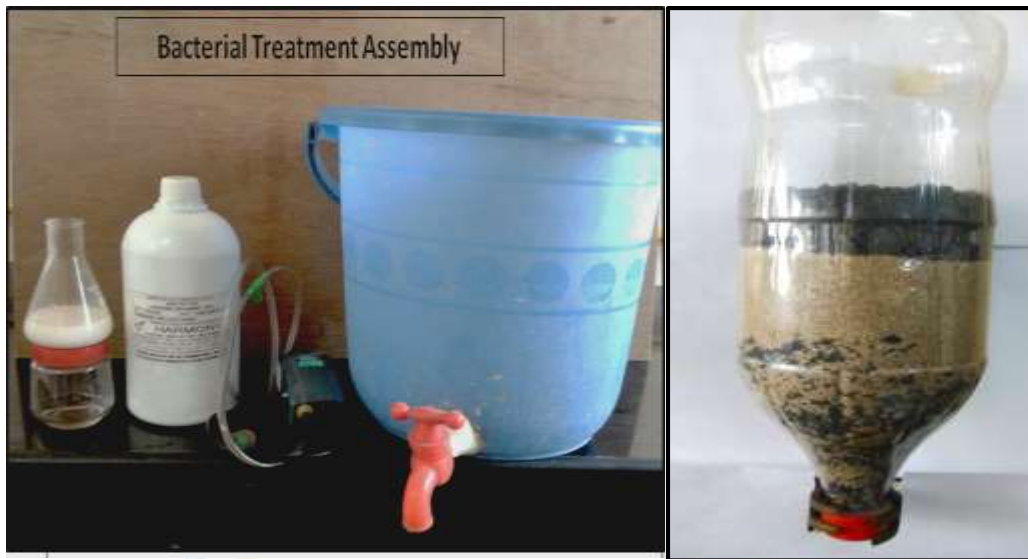
Key: From L to R- Antifoaming agent, sparger, treatment chamber & carbon and sand filter.
