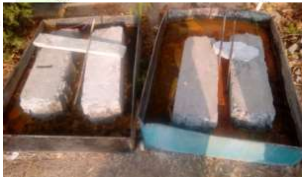
Fig.6 Accelerated corrosion process setup.
