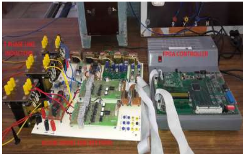
Fig. 4.4.1. Hardware prototype of Active Front End Rectifier
