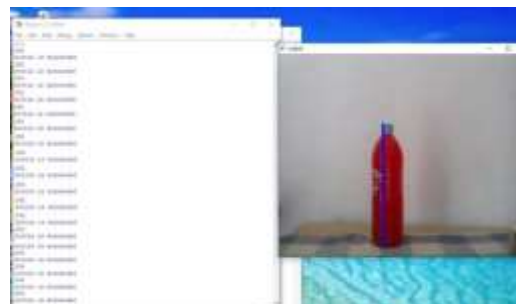
Fig8: Simulation results when filled to undesired level i.e., the bottles are discarded
