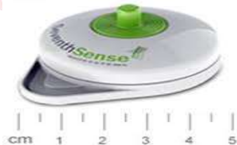
Fig 3.4.1: Seventh Sense Bio-systems TAP 20™ Painless Blood Draw Device
