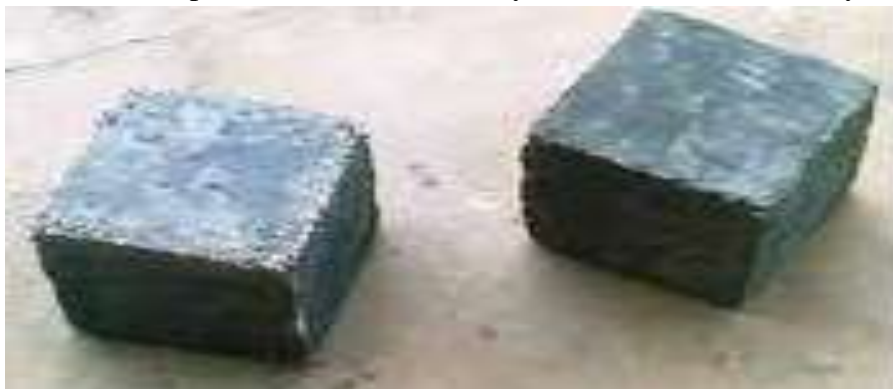
Figure1: Cube prepared with normal concrete
