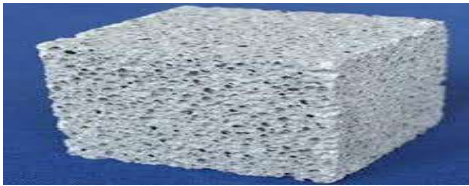
Figure2: Cube prepared with light weight aggregate
