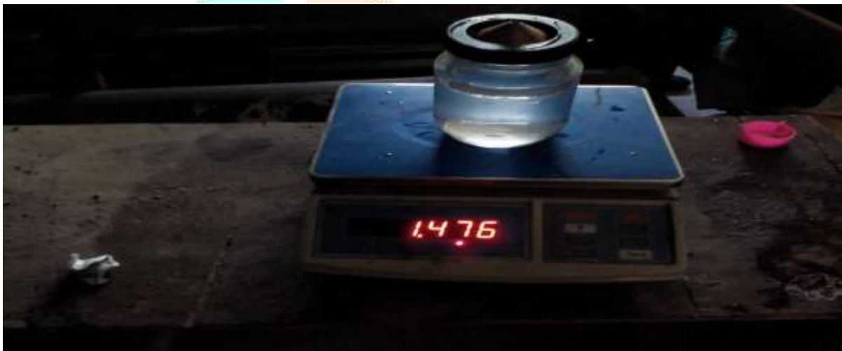
Fig – 3.3. Specific Gravity on Fine Aggregate
