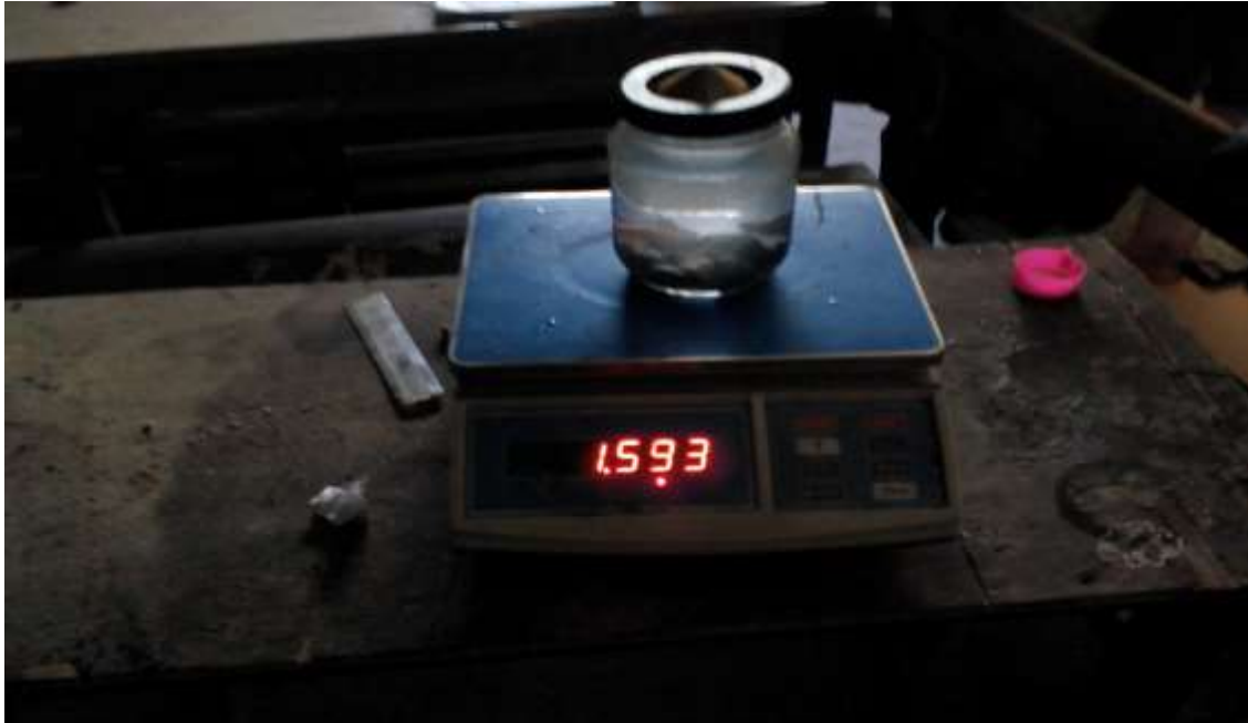
Fig 3.3 Specific Gravity on Coarse Aggregate
