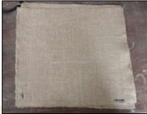
Fig. 2 Jute fabric cut in sheets of 30 \times 30 \text{ cm}^2
