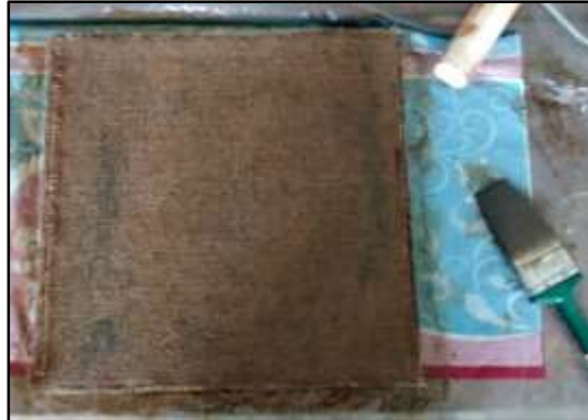
Fig. 4 Manufactured specimen of Jute fiber reinforced phenolic composite with 5% of SiC
