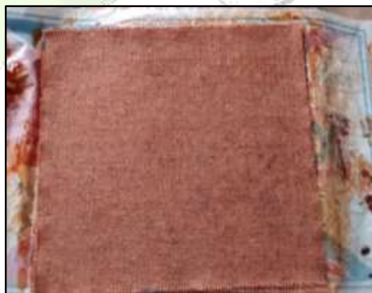
Fig. 3 Manufactured specimen of Jute fiber reinforced phenolic composite with 0% of SiC
