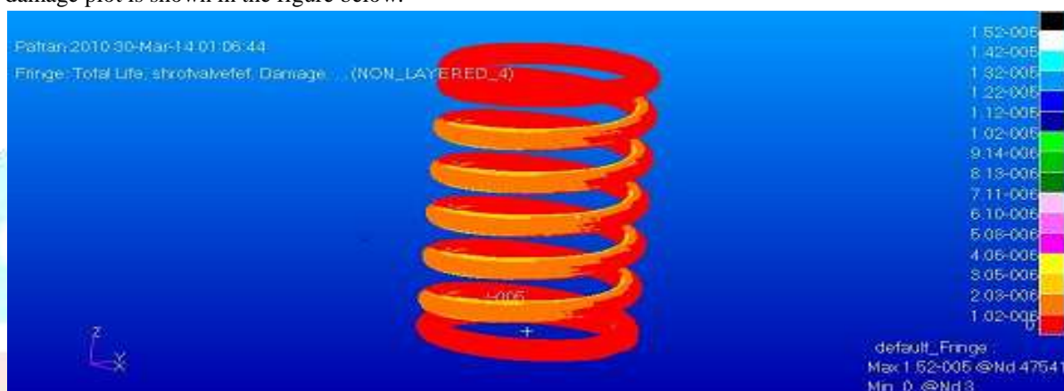
Figure 10 Damage plot of compression spring
