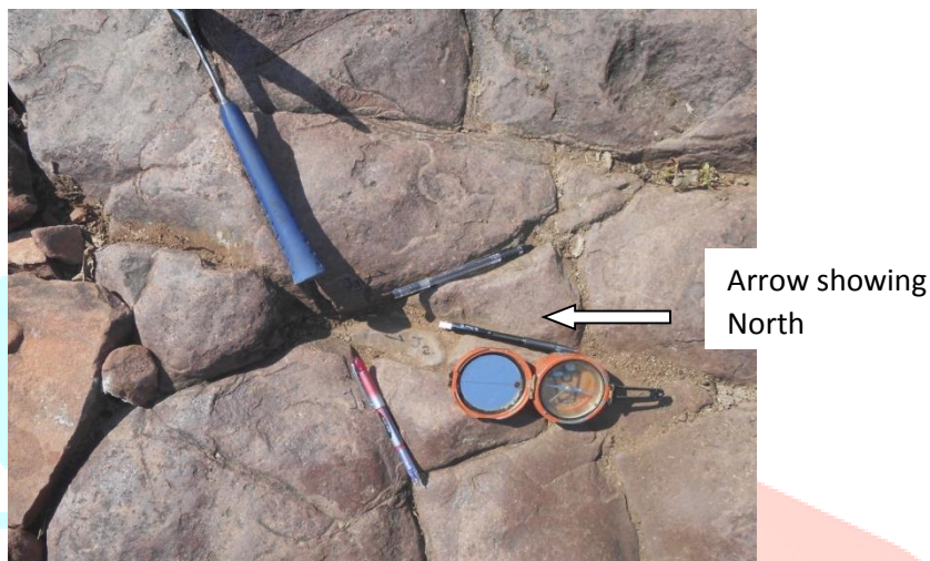
Fig 16 Planar view of three set of joints in Jarara hill, Trend shown by pen, hammer and brunton compass
