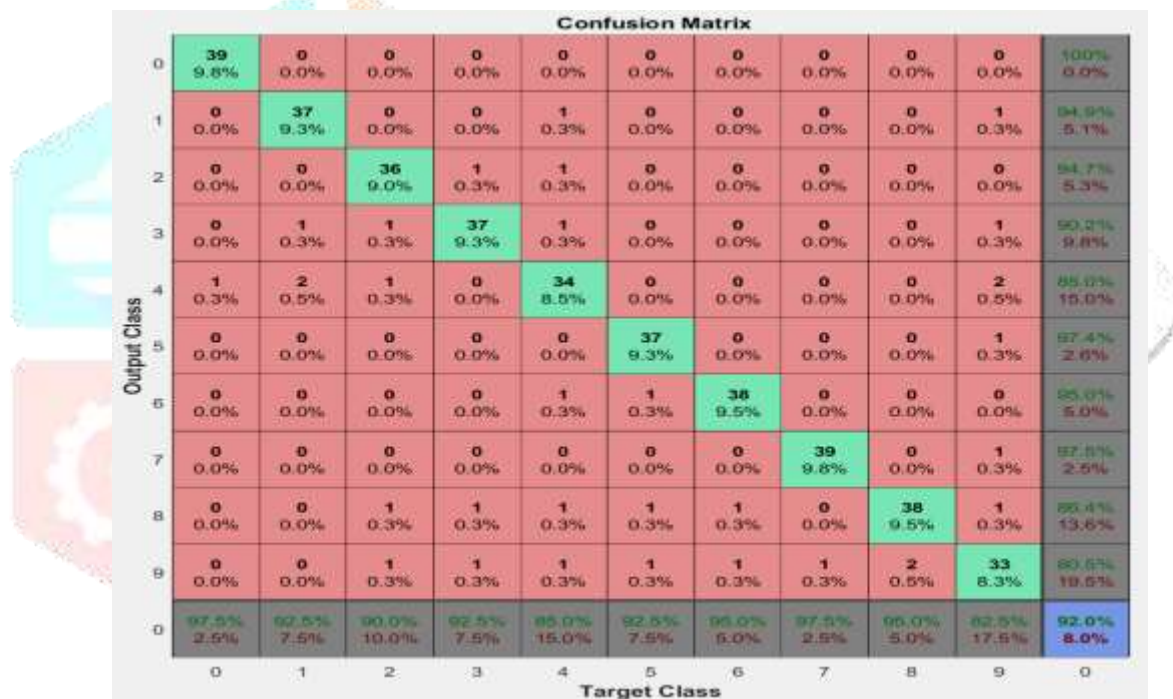
Figure 6.1: Confusion matrix using fusion of HOG and zoning features and SVM on Chars74K benchmark numeric data set.
