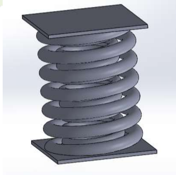
Figure 2: 3D model of the concentric helical coil spring
