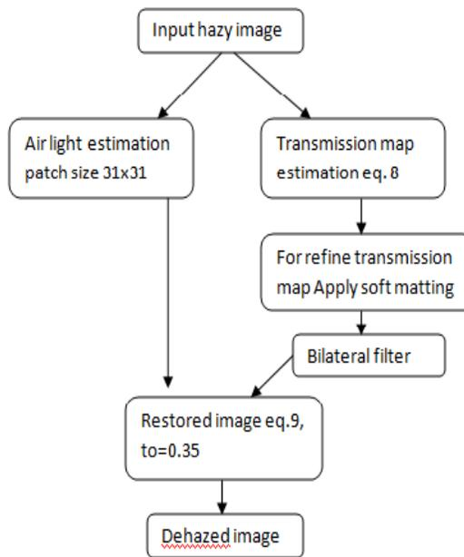
Fig 4: Block diagram for IDCP algorithm
