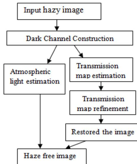
Fig2. Basic block diagram of DCP based dehazing algorithm
