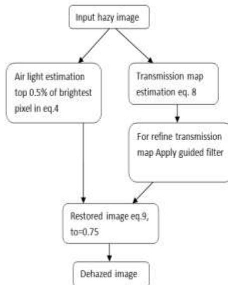
Fig 5: Block diagram for IDCP with guided filter algorithm.
