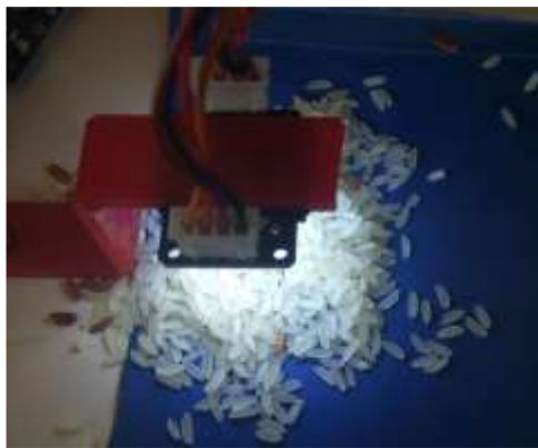
Figure 3.5 Normal Rice Sensing and Display of normal rice indication in LED display
