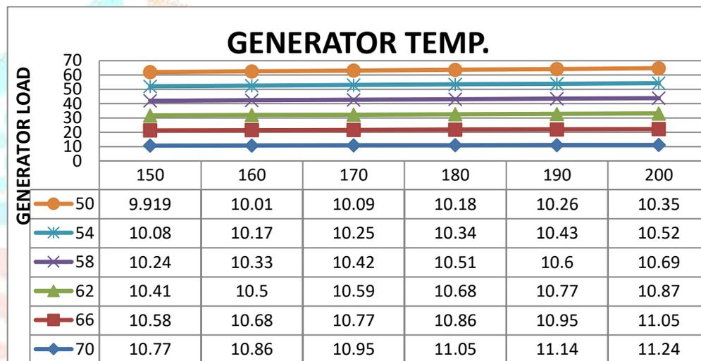
Fig. 8 Generator load vs. generator temperature for different condenser temperature
