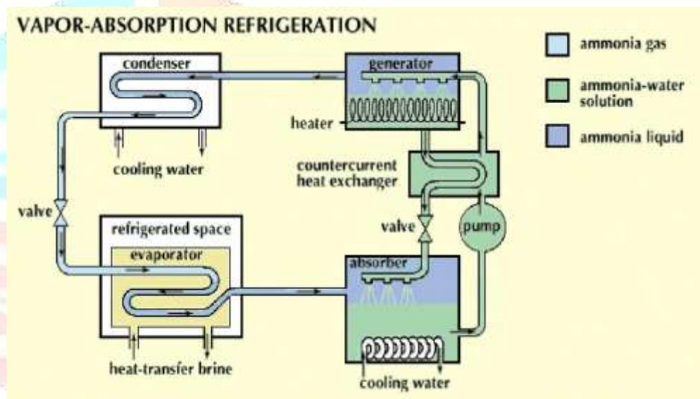
Fig. 3 Ammonia – water based VAR system cycle
