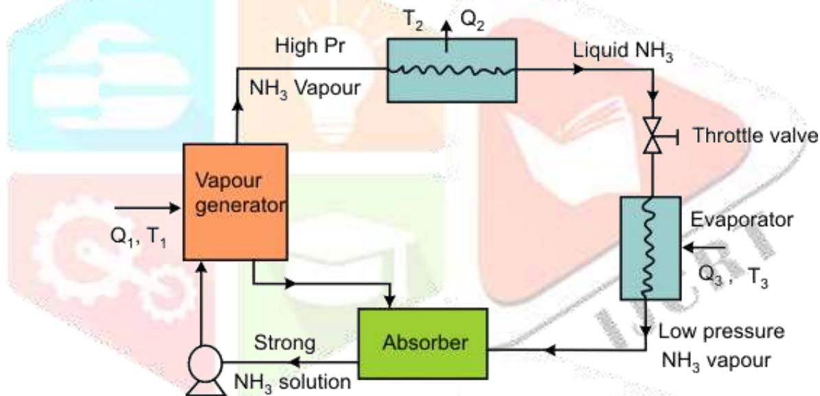
Fig. 2 Vapour absorption refrigeration cycle
