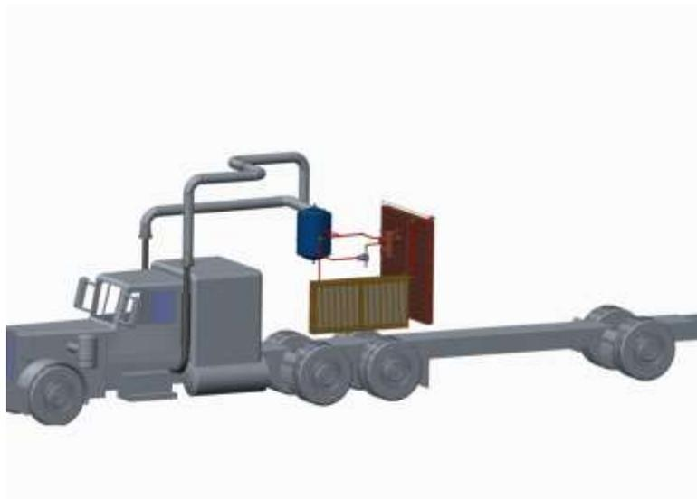
Fig. 5 VAR system truck chassis
