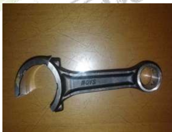
Fig.3.2 Connecting rod after failure
