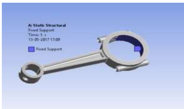
Fig. 4.1 3D model of connecting rod
