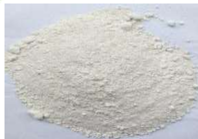
Fig 2 Egg shell Powder used in Concrete
