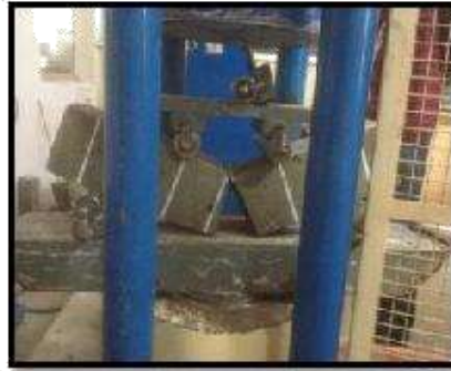
Fig 4 Split Tensile Strength Test
