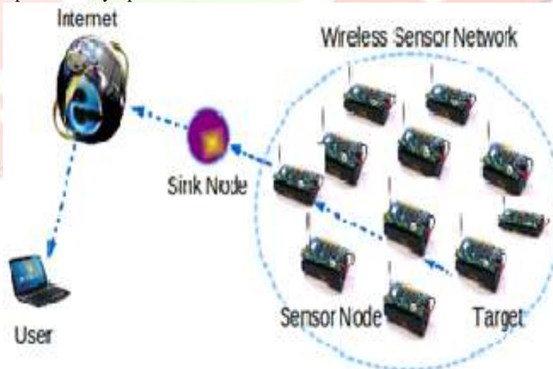
Figure 1: Wireless Sensor Network
