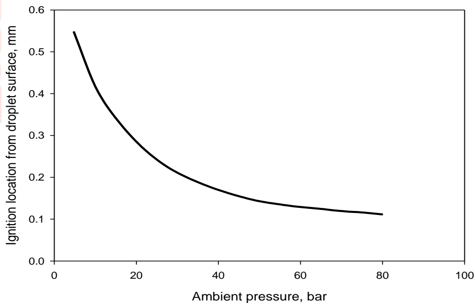
Figure: 5 Variation of ignition location with ambient pressure at ignition for a droplet of initial diameter 0.5 mm.
