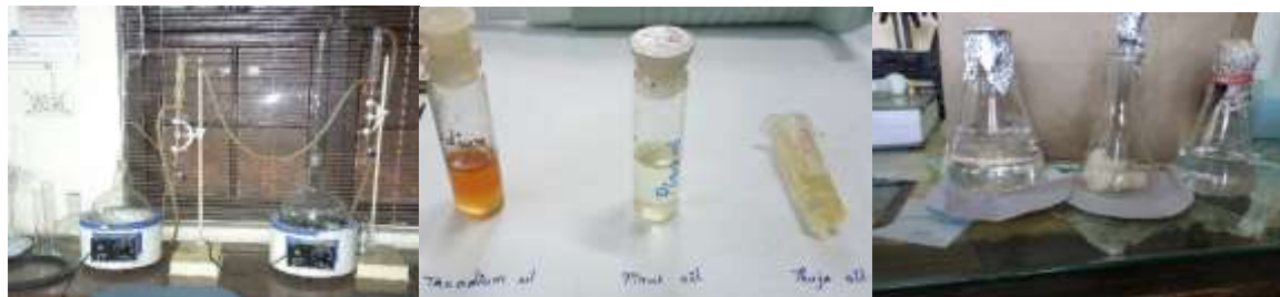
Fig.2a. Clevenger type apparatus. Fig.2b. Extracted oils Fig.2c. DDW and saline media.
