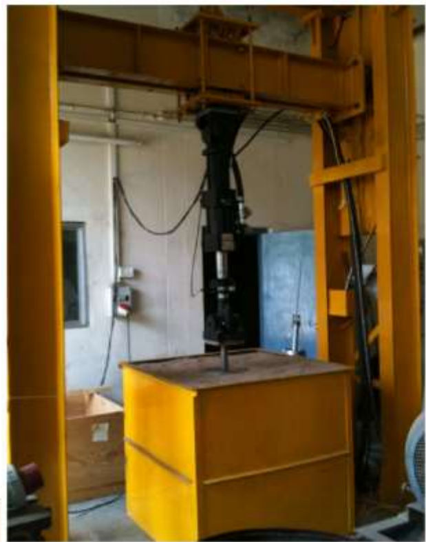
Fig. 3 Test tank and the loading system used in the study
