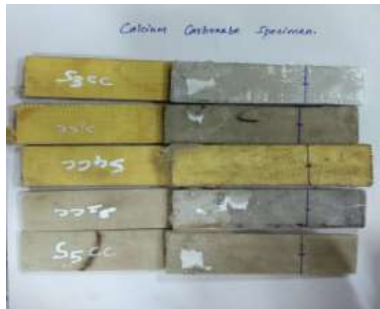
Fig 10. CALCIUM CARBONATE FILLER LAP JOINT
