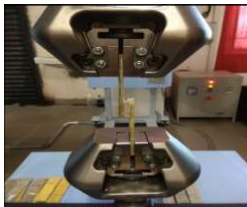
Fig 12. BREAKING OF SPECIMEN IN UTM
