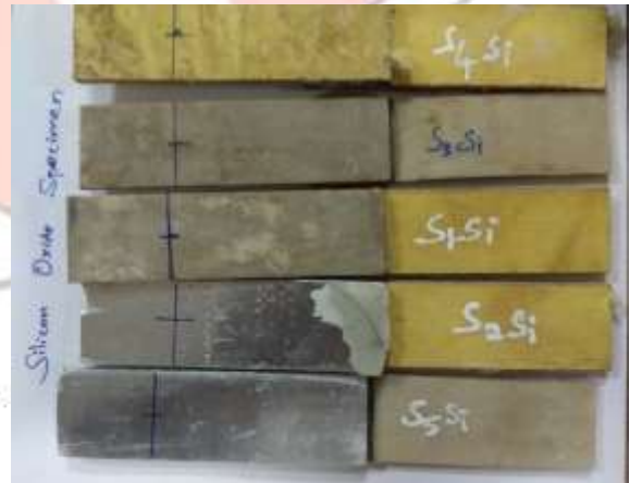
Fig 9. SILICON DIOXIDE FILLER LAP JOINT
