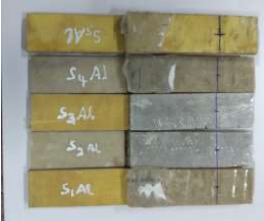
Fig 8. ALUMINIUM FILLER LAP JOINT
