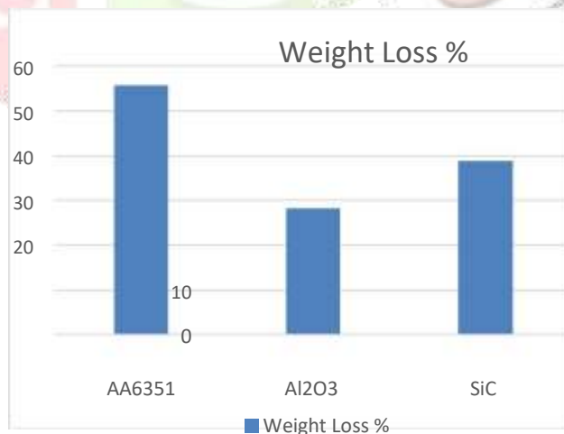
Fig. 9 Comparative wear mass loss chart for 10N load
