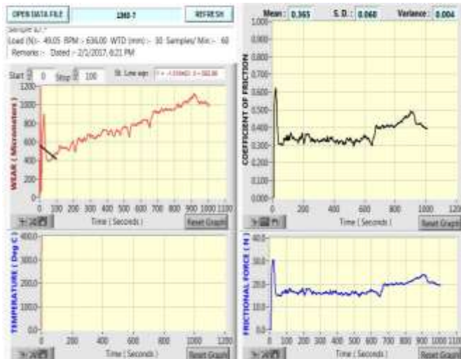
Fig.8. Wear rate under 50N load for AA6351/SiC/Gr specimen Table. 3 Comparison of Weight loss% of Pins of Three Specimens
