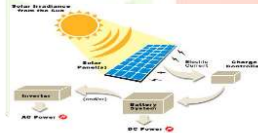
Fig. 3. Solar panel system
