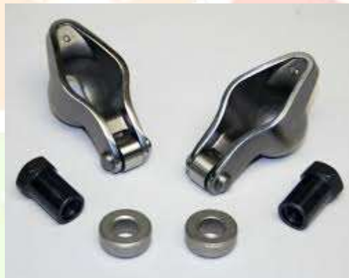
Fig 3: Roller tipped rocker arm
