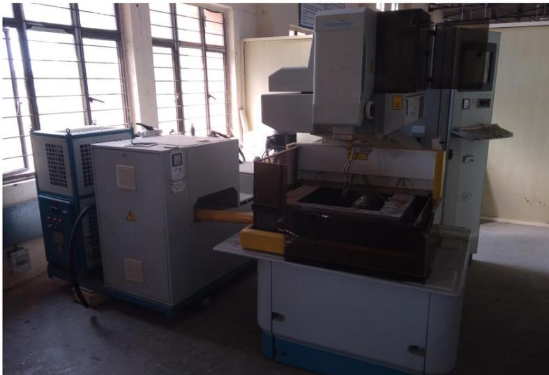
Figure-1: CNC Electro Discharge machine sprincut
