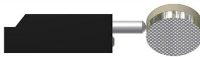
Fig: 2 Diamond burnishing tool
