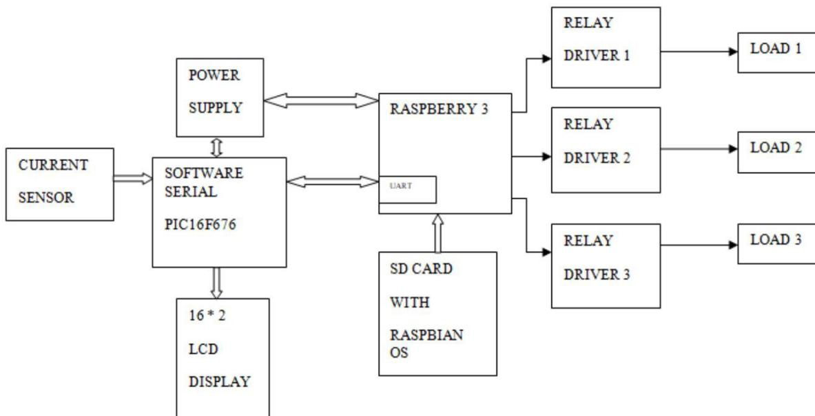
Fig 3.1 Proposed Block Diagram
