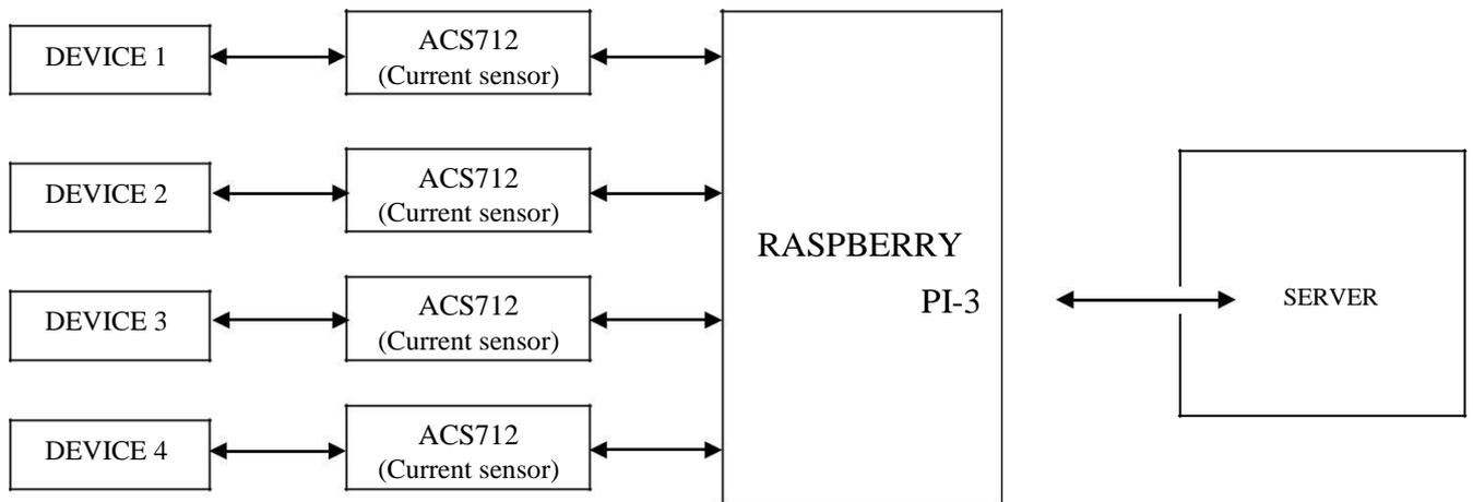
Fig 2 Existing Block Diagram
