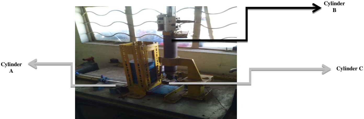
A model of embossing machine
