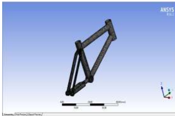
(Fig-2: Meshed model of bicycle frame)
