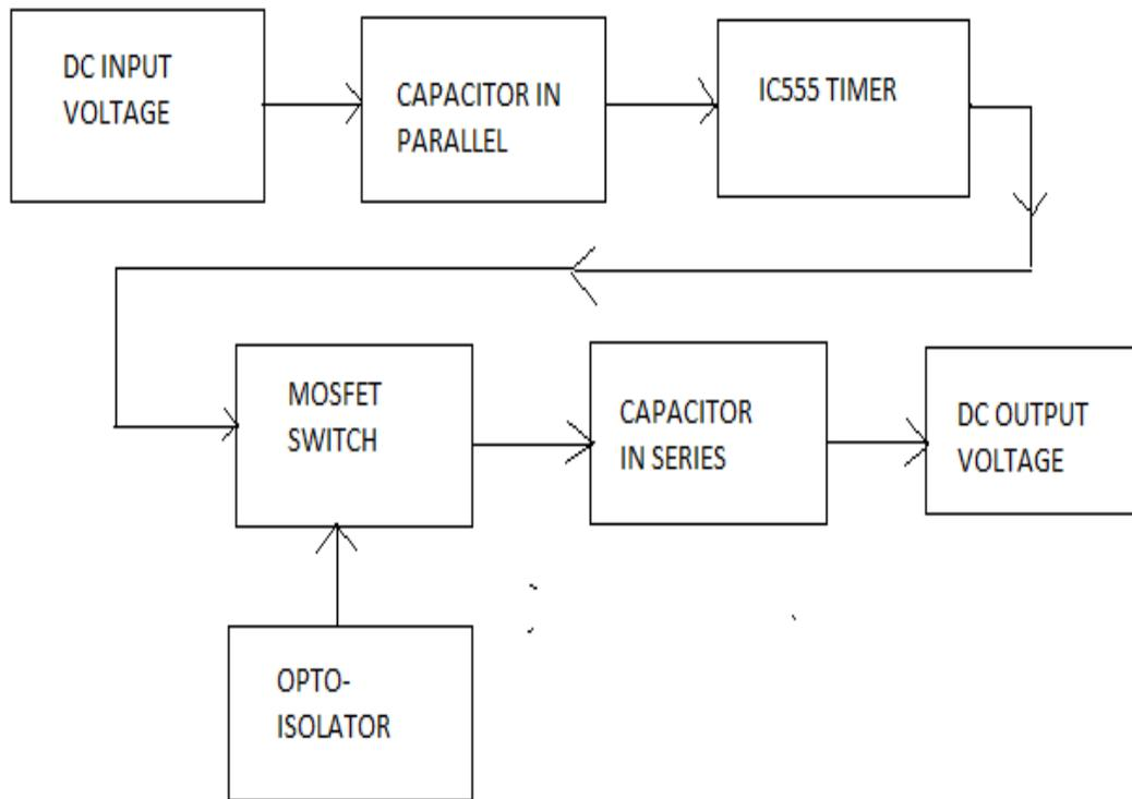
FIG.3: BLOCK DIAGRAM OF GENERATION OF HVDC USING MARX GENERATOR [2]
