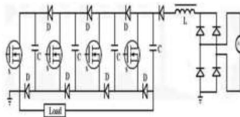
Fig.2: Contemporary Structure of Marx Generator
