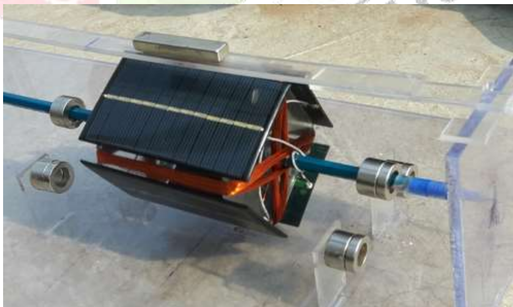
Figure 7-Final Assembly of motor
