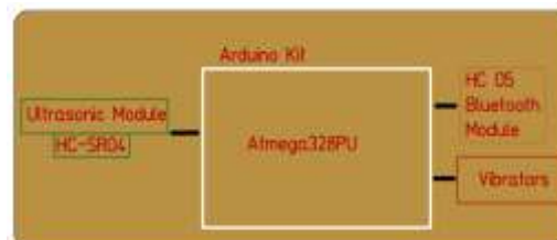
Figure 1 Internal Block Diagram of System
