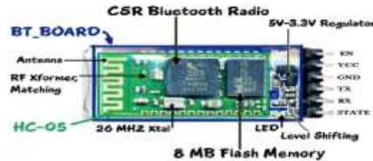
Figure 5 HC-05 Bluetooth Module
