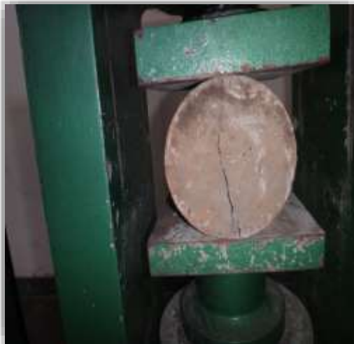
FIG: TESTING OF SPLIT TENSILE STRENGTH OF CONCRETE
