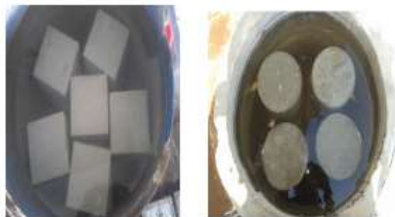
CURING OF CONCRETE CUBES & CYLINDERS
