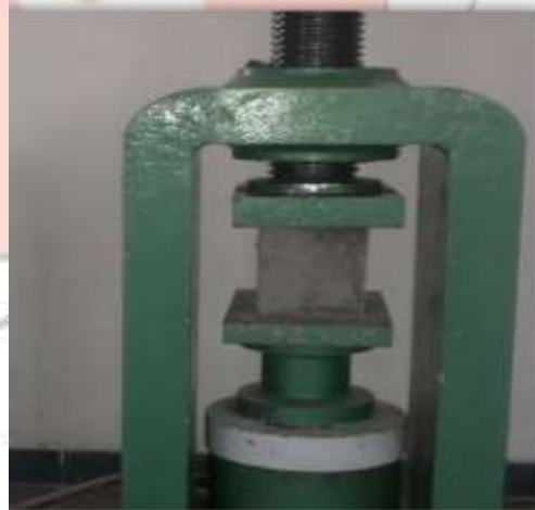
FIG: TESTING OF COMPRESSIVE STRENGTH OF CONCRETE (CTM)
